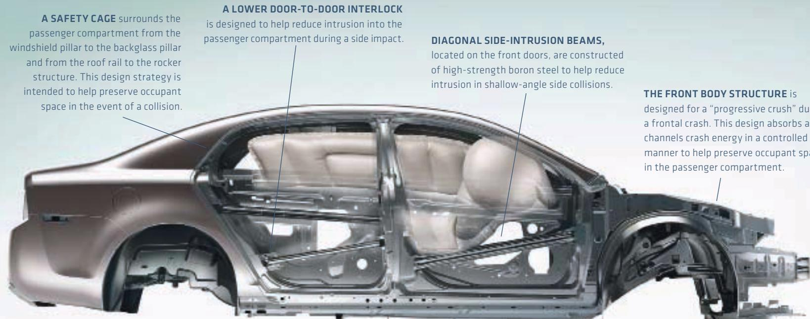
**A SAFETY CAGE** surrounds the passenger compartment from the windshield pillar to the backglass pillar and from the roof rail to the rocker structure. This design strategy is intended to help preserve occupant space in the event of a collision.
