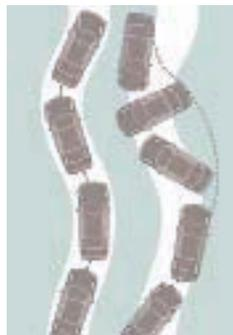
The Stabilizer Trak Electronic Stability Control System helps you stay the course by detecting the difference between the steering wheel angle and the direction the vehicle is actually turning. It then uses the brakes and, if necessary, adjusts engine torque to help you keep your vehicle on your desired track.
